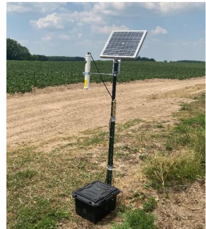
Fig. 1. Rotating arm impactation sampler deployed in a commercial potato field in 2023.
